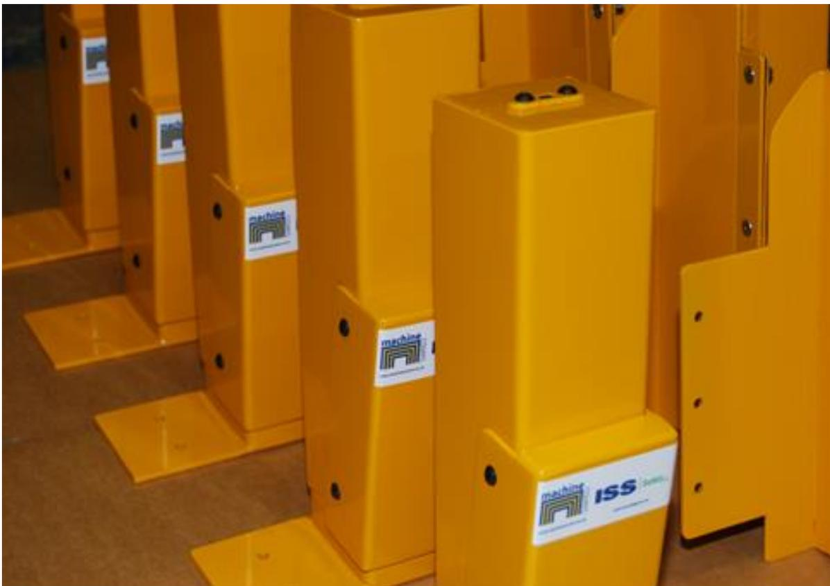
Colchester fitting kits 24638c for lathe tray fixing shown above (optional and not included with standard AR boxed roller unit supply)
