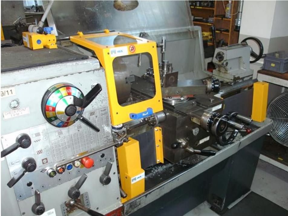
The picture above details a fully compliant Colchester lathe that meets all of the requirements laid out in the current C standards for a manually operated lathe.
