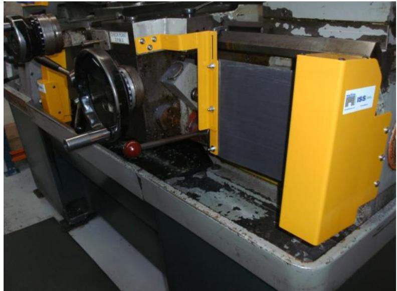
Colchester fitting kits 24638c for lathe tray fixing shown above (optional and not included with standard AR boxed roller unit supply)
